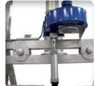
Fan and tension cylinder ensure big bag pre-forming and internal shaping
