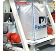
Vibrating table provides a compacted material by means of vibration ensuring a maximum of volume reduction of the material in the big bag
