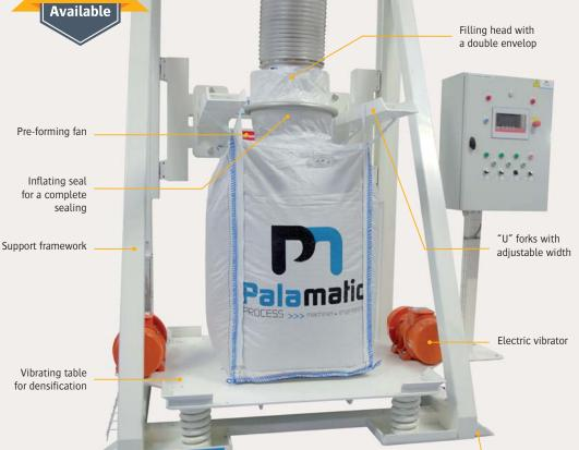
The whole adjustable structure provides flexibility to accommodate a range of bag
