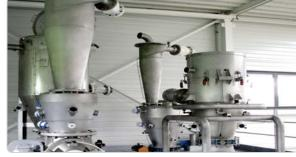
Pneumatic conveying equipment: pressure, vacuum, dilute or dense phase
