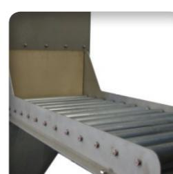
Roller conveyor to feed the machine
