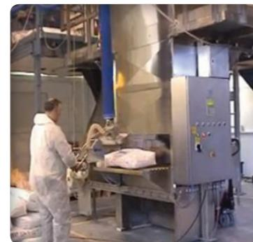
► Feeding of the machine with a tube lifter for sacks
