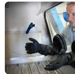
➤ Glove box for handling product in a closed and contained area: glass and gloves
