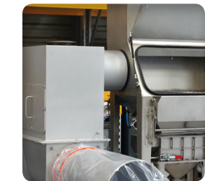
➤ Side discharge chute for the bag to maintain a clean working area and to eject the "dirty" emptied sack in a contained area
