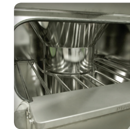
➤ Mirror-polished finishes to improve product flow and hygiene. Particularly suitable to the pharmaceutical industry
