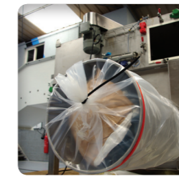
▶ Screw compactor for the evacuation of the emptied sacks and the reduction of dust emissions
