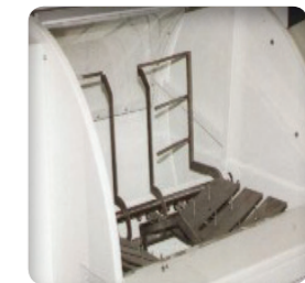
▶ Ejection of empty bags into the compactor
