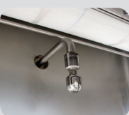
Rotative cleaning nozzles/heads - Clean In Place (CIP)
