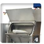
Access door mounted on gas spring: an accompaniment to the opening and
