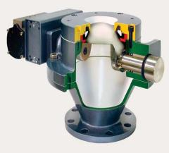
Abrasive materials: abrasive slurries, powders, bulk granules and gases loaded with dust cause erosion of the seat and the inefficient closure of classic valves. The inflatable seal and its function of automatic compensation overcomes the problems related to wear because of abrasive materials.
