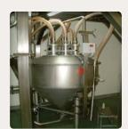
Vacuum pneumatic conveying with inte grated «weight gain» scale. This pattern is specially designed for the suction of multi-components
