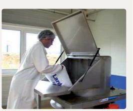
Structure and parts in contact with the material: mild steel, 304L Access door: plexiglass, antistatic lexan, tempered laminated glass **Sealing:** EPDM, NBR, natural rubber Finishes: customized RAL, peening, electropolishing
