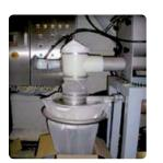
Conditioning unit at the output of an though screw conveyor
