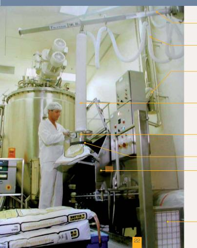
Triangular post mounted jib crane to provide a lifting stroke of 1,700 mm (overhead room 3m.)
