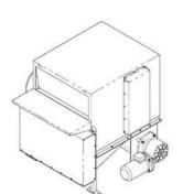
The SAS® bag dump system allows, due to its mode of operation, the deconditioning of explosives material with a very low or low EMI. The moving parts included in the SAS provide slow speeds, thus avoiding the risks of sparks caused by impacts.
