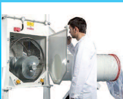
Sack compactor integrated with an automated sack opening machine
