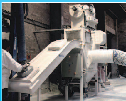
Sack compactor integrated with an automated sack opening machine
