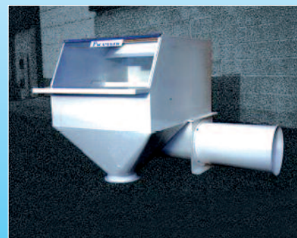
Sack compactor integrated with a manual sack opening machine
