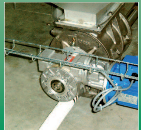
All stainless steel valve for pneumatic transfer of granulated plastic from storage silos
