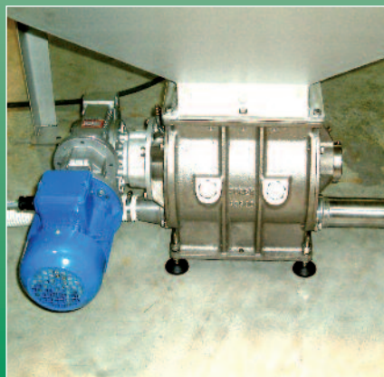
All stainless steel valve for pneumatic transfer of granulated plastic from storage silos
