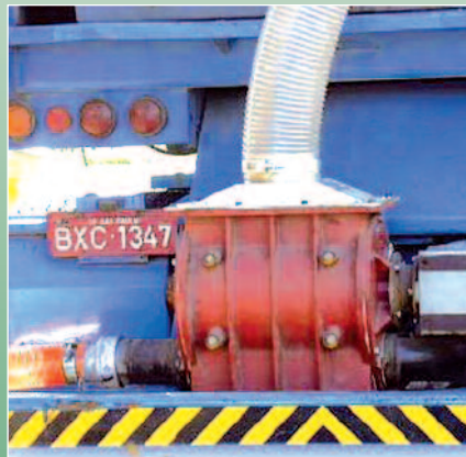
Valves at the blower lorry outlet
