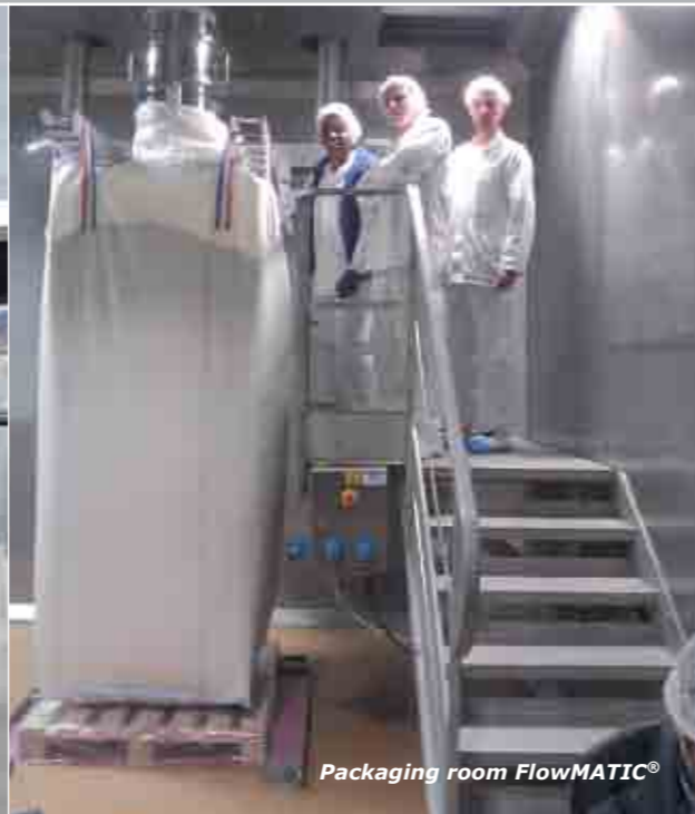
Hopper fitted with CIP and inspection door
